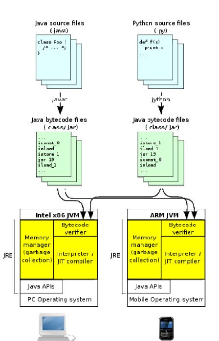
Source code is compiled to Java bytecode, which is verified, interpreted or JIT-compiled for the native architecture. The Java APIs and JVM together make up the Java Runtime Environment (JRE).
