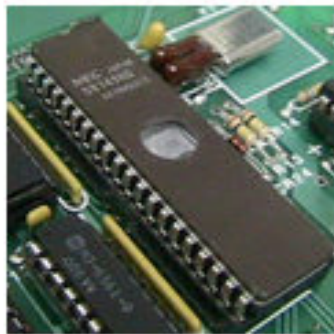
This 8749 Microcontroller stores its program in internal EPROM
