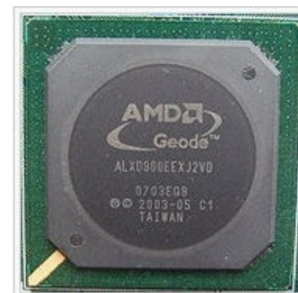
AMD Geode is an x86 compatible system-on-a-chip
