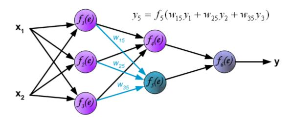
Propagation of signals through the output layer.
