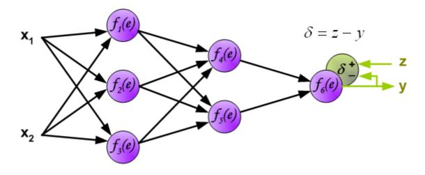
It is impossible to compute error signal for internal neurons directly, because output values of these neurons are unknown. For many years the effective method for training multiplayer networks has been unknown. Only in the middle eighties the backpropagation algorithm has been worked out. The idea is to propagate error signal d (computed in single teaching step) back to all neurons, which output signals were input for discussed neuron.
