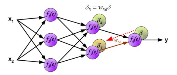
The weights' coefficients  $w_{mn}$  used to propagate errors back are equal to this used during computing output value. Only the direction of data flow is changed (signals are propagated from output to inputs one after the other). This technique is used for all network layers. If propagated errors came from few neurons they are added. The illustration is below:
