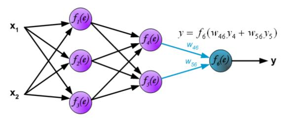
In the next algorithm step the output signal of the network *y* is compared with the desired output value (the target), which is found in training data set. The difference is called error signal *d* of output layer neuron.
