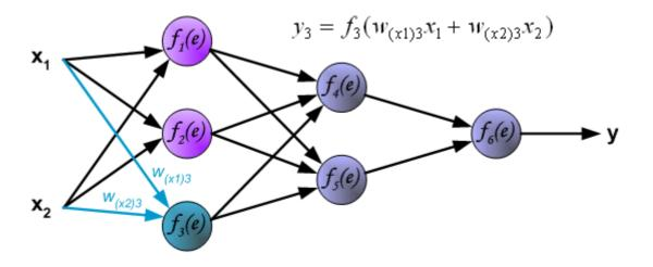
Propagation of signals through the hidden layer. Symbols  $w_{mn}$  represent weights of connections between output of neuron m and input of neuron n in the next layer.
