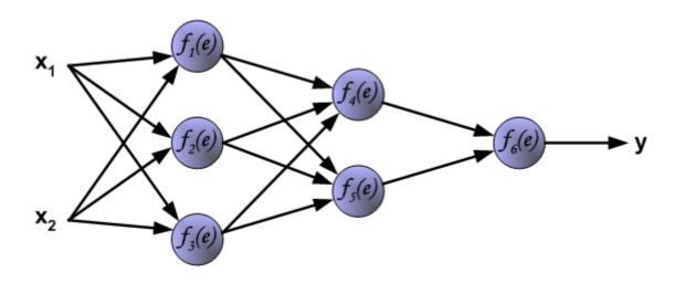
Each neuron is composed of two units. First unit adds products of weights coefficients and input signals. The second unit realise nonlinear function, called neuron activation function. Signal e is adder output signal, and y = f(e) is output signal of nonlinear element. Signal y is also output signal of neuron.
