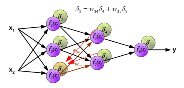
When the error signal for each neuron is computed, the weights coefficients of each neuron input node may be modified. In formulas below df(e)/de represents derivative of neuron activation function (which weights are modified).
