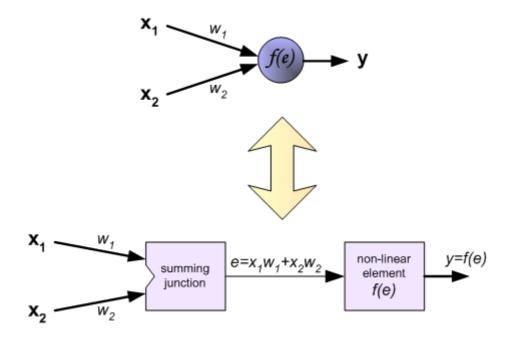
To teach the neural network we need training data set. The training data set consists of input signals  $(x_1 \text{ and } x_2)$  assigned with corresponding target (desired output) z. The
